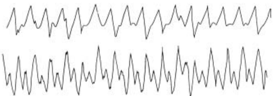
図-4 (b)  $U=2.84 \text{ m/s}$  (Mixed or 2nd order locking)
