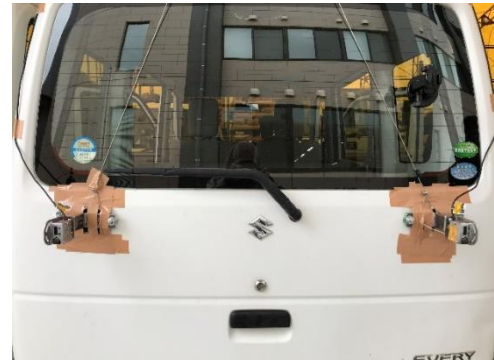
Figure 3 Example of simple laser sensor placed at back of car.
