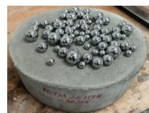
Figure 3: Specimen with abrasive charges placed on the surface
