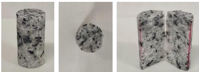
Fig.1 Granite specimen including tensile single fracture
