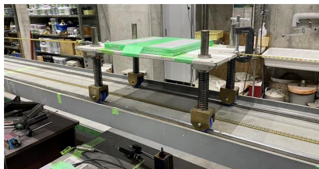
Fig. 1 In-house experiment on a model bridge under a moving vehicle.
