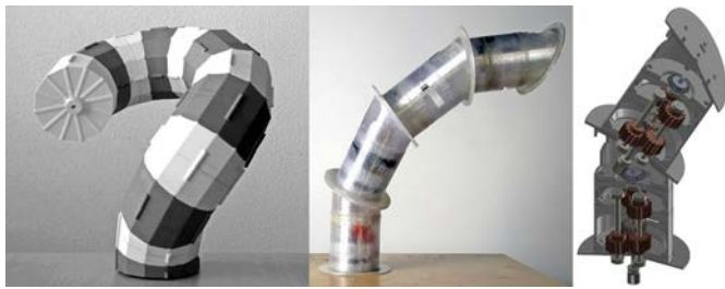
Fig. 3 Left: 3D-printed mock-up of a dodecagonal 12 module Arm-Z. Middle: An early prototype of a 4-unit Arm-Z. Right: Isometric cutaway showing the drive for rotation which is carried by the gear system.
