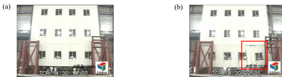
Fig. 1 Screenshot of the video data: (a) nominal state; (b) with cracks
