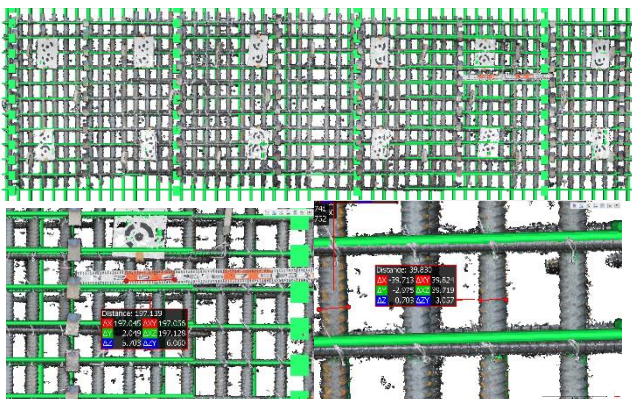
Fig. 5 photogrammetry model superimposed on 3D CAD model
