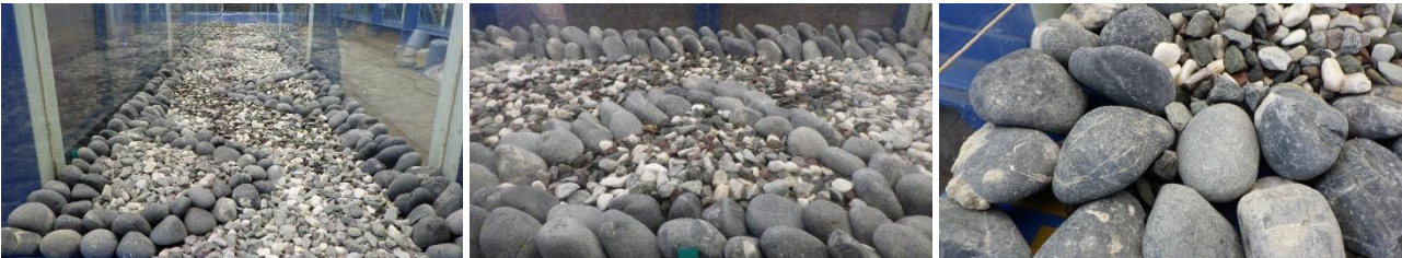
Photo 1 Left (a): Improved gravel mounts' model viewed from downstream. Centre (b): a gravel mounts shown from the left side wall. Right (c): closer look at the stacked boulders around the gravel mounts (viewed from downstream).
