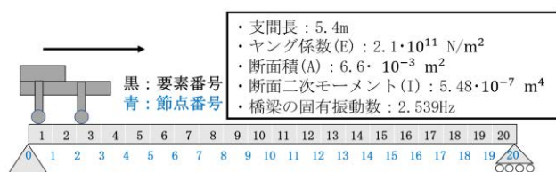
Fig.1 Beam model for simulation with mechanical properties.
