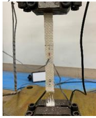
Fig.6 Morphology of Al specimen fracture
