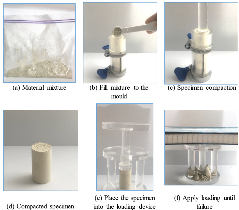
Fig. 2 Specimen preparation process
