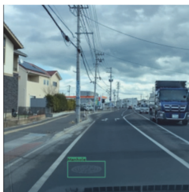
Step1 Manhole detection by object detection
