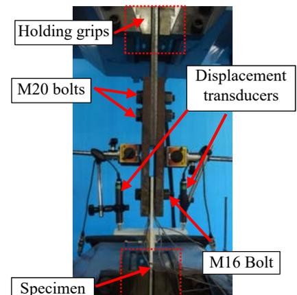
Fig. 2. Experimental setup
