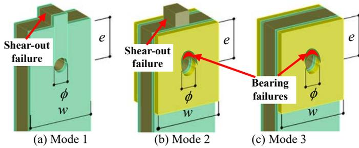
Fig. 3. Three types of failure modes
