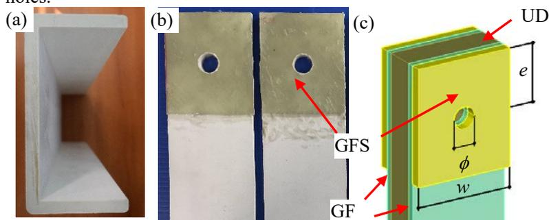
Fig. 1. GFRP connections. (a) original shape, (b) GFRP plates with GFS strengthening, (c) connections configurations.
