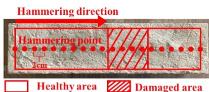
Fig. 2 Concrete sample
