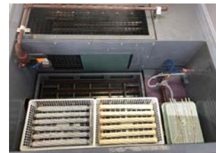
Fig.2 Accelerated corrosion method
