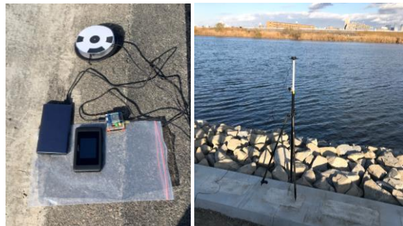
Figure.3 RTK-GNSS system on the right picture with a Wi-Fi router and battery, antenna connected to the system in the right picture.
