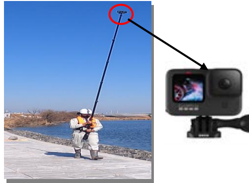
Figure.2 5.5 Meters pole and GoPro Hero9 attached to the end The software used for 3D modeling is Agisoft Metashape Professional which is used for dense point cloud generation and editing, 3D modeling, digital elevation model generation. The software used for referencing the 3D models with RTK-GNSS GPS data is Cloudcompare software which is an open-source software used mainly for post-processing purposes.
