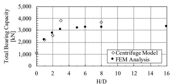
Figure 2. Dense sand layer thickness vs. bearing capacity
