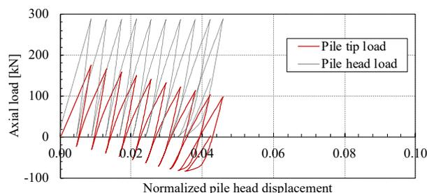
Figure 3. Pile tip load vs. pile head displacement for Case 8D (CLT1)
