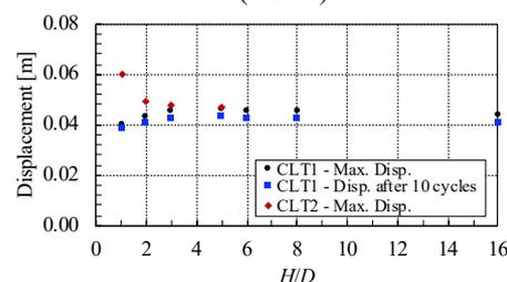
Figure 4. Pile head displacement (maximum and after 10 cycles)
