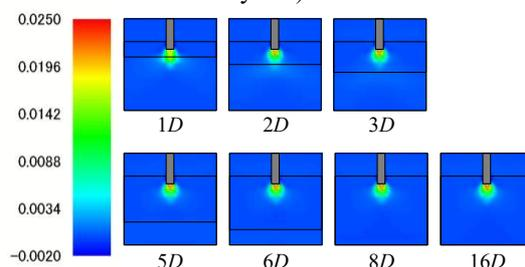
Figure 5. Volumetric strain in soil surrounding pile tip after 10 cycles (CLT1)
