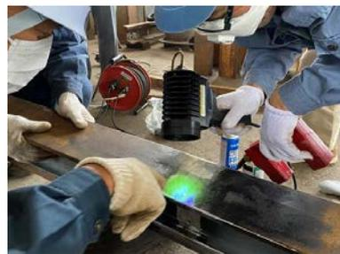
写真-8 磁粉探傷検査
