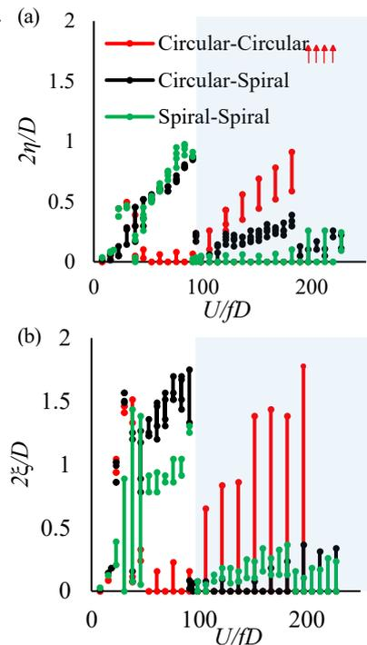
Fig. 3 Free vibration responses of downstream cable in (a) vertical and (b) horizontal direction
