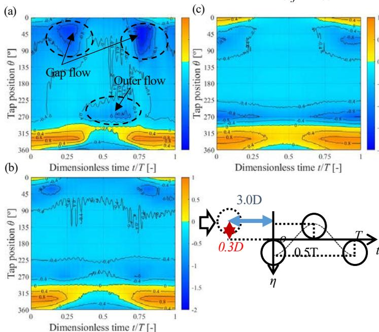
Fig. 6 Time series  $C_p(t)$  of downstream cable in one period  $T$  of the forced vibration
