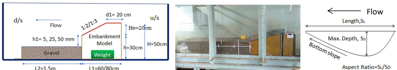
Figure-1: Schematic diagram (left), Image of experimental setup at laboratory (middle) and Typical scour hole (right)
