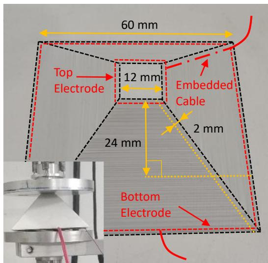
Fig.3 Pyramid unit and experiment setup
