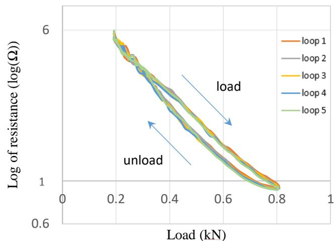
Fig.4 Compression test of a pyramid unit
