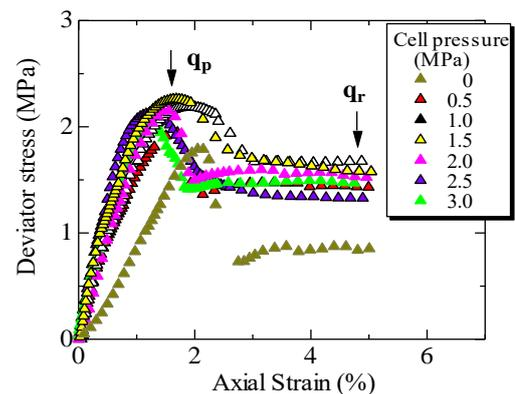
Fig. 3 Stress-strain relationship in triaxial UU
