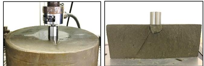
(a) Water floating during the test (b) Wedge formed under the footing
