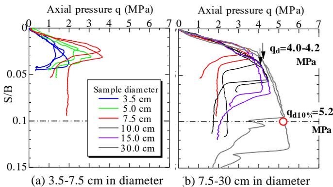
Fig. 5 q-S/B curve of bearing capacity test
