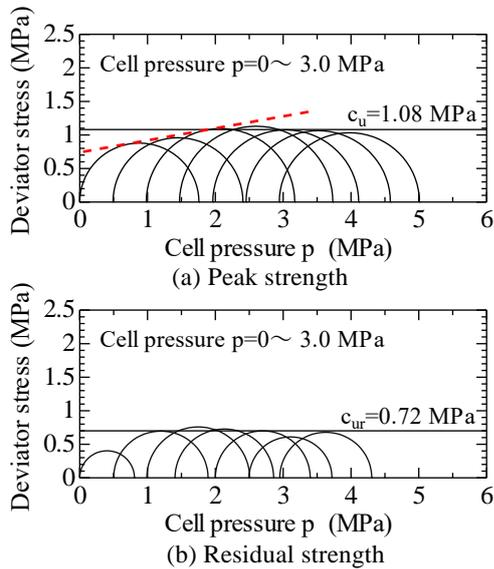
Fig. 4 Mohr's circles for triaxial UU
