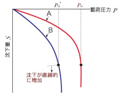
Fig. 6 Determination method for the  $q_d$
