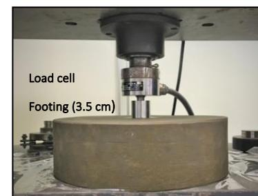
Fig.2 Test specimens 30 cm diameter
