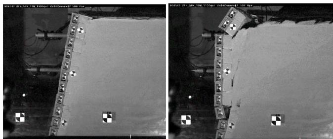
図5 1000gal(変位200mm) 図6 1100gal(変位630mm)
