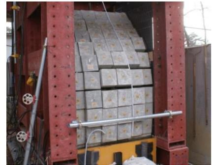
図1 石積み壁載荷試験の様子<sup>1)</sup>
