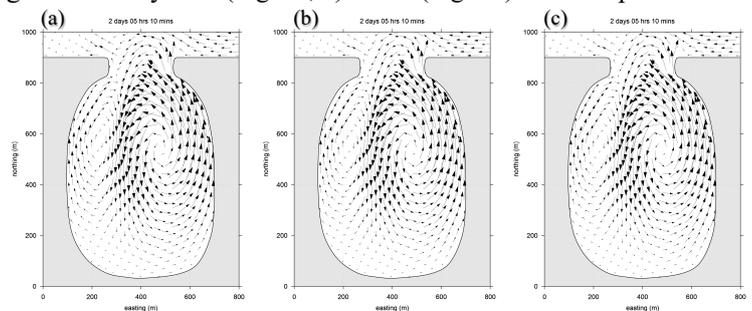
Fig. 2 Snapshot of flow patterns at high tide, (a) Case 1, (b) Case 2, 10 layers, (c) Case 3
