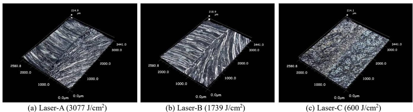
Fig.1 Surface of laser-treated carbon steel plate
