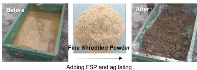
Figure 2. Treatment of mud with high water content using FSP (Sawamura et al., 2017).
