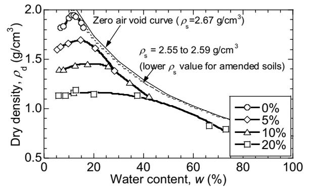
Figure 6. Compaction curves mixtures.
