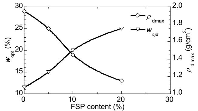
Figure 7. Variation trend of optimum water content and maximum dry density to FSP content.
