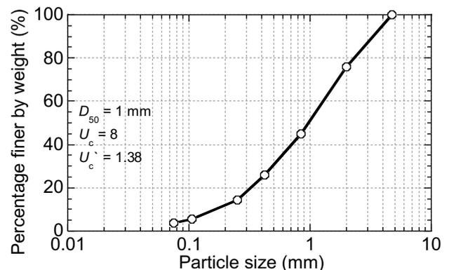
Figure 4. Particle size distribution curve of soil.
