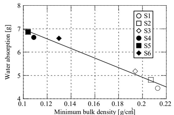
Figure 3. Relation of water absorption capacity to minimum bulk density of soil (Sawamura et al., 2017).
