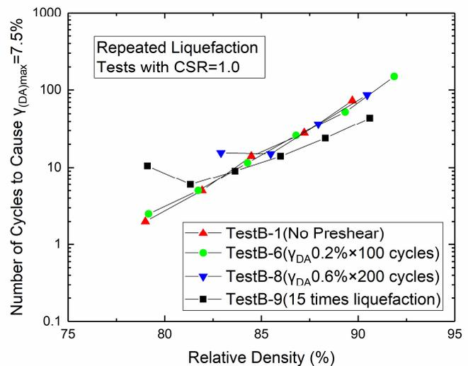
Fig. 5 Relationship between relative density and number of cycles to reach  $\gamma_{DAmax}$  of 7.5%
