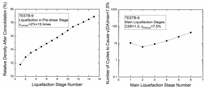
Fig. 4 Density change in pre-shear stages (left) and number of cycles to reach  $\gamma_{DAmax}$  in main liquefaction stages (right) of Test B-9
