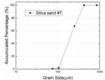
Fig. 1 Grain size distribution of silica sand #7
