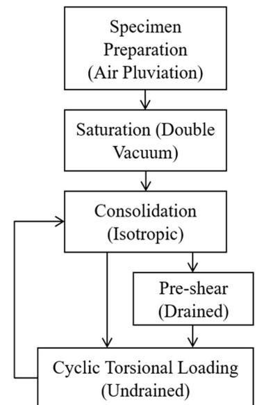
Fig. 2 Flow chart of the test
