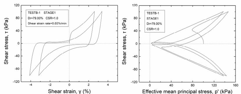
Fig. 3 Stress-strain relation (left) and effective stress path (right) of test without pre-shear
