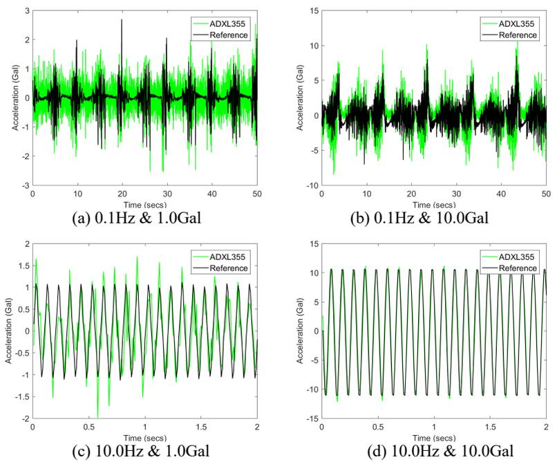
Fig. 4. Acceleration waveform comparison
