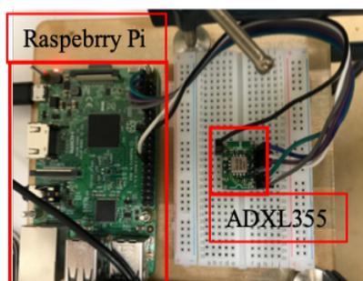
Fig. 1. Wiring demonstration
