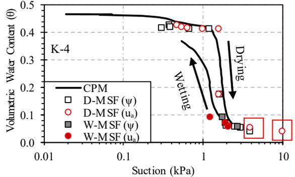
Figure 4: K-4 sand SWCCs. Solid line represents the CPM results while the plots represent the MSFM
