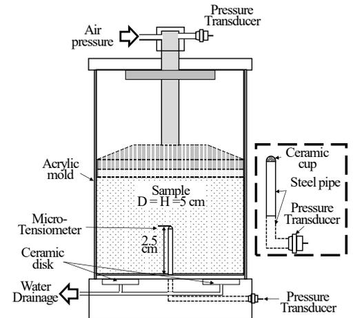
Figure 1: CPM cell (schematic).
