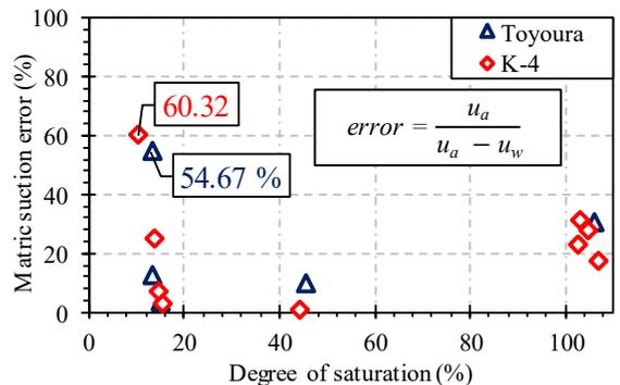
Figure 6: Error associated with the matric suction utilizing the conventional MSFM
