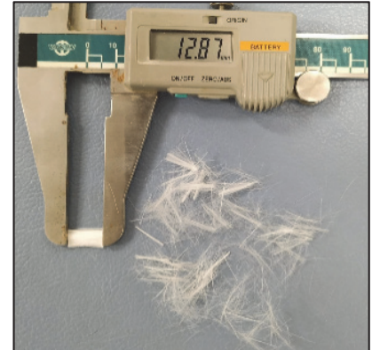
Photo 1. Polypropylene fibers used in this study
