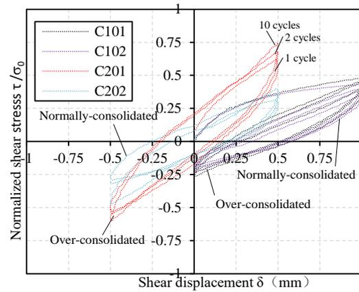
Fig. 3. Cyclic shear stress - displacement behavior under one-sided and two-sided shearing
