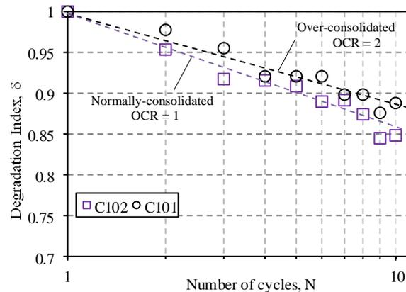
Fig. 4. Degradation index of cyclic shear stress in the one-sided shearing
