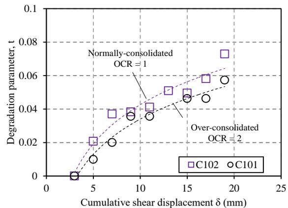
Fig. 5. Degradation parameter of cyclic shear stress in the one-sided shearing
