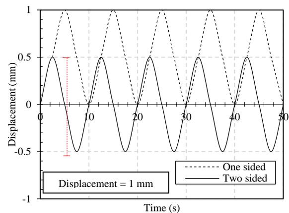
Fig. 1. Schematic of (one-sided and two-sided) cyclic loading.
