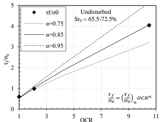
Fig. 2. Relationship of normalized shear stress and OCR.
