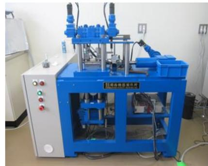
Fig.1 Constant stress direct shear
