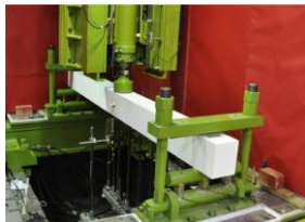
Photo 1 Test setup for fall-weight impact loading.
