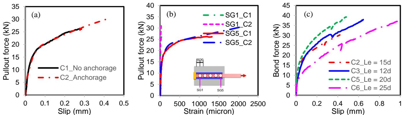
Fig. 2 Comparison in bond and strain responses between the cases with and without anchorage, and effect of ETS bar diameter
