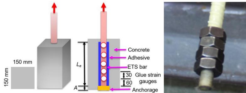
Fig. 1 Configuration of the tested specimens and the anchorage device (anchoring nuts) at end of GFRP bar
