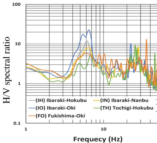
Fig. 2. H/V spectral ratio of 5 events recorded at PBT in Oya.
