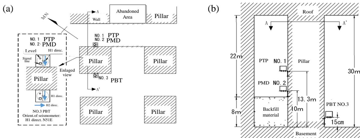
Fig. 1. Layout of underground quarry and locations of instruments, (a) plan view, (b) side elevation view.
