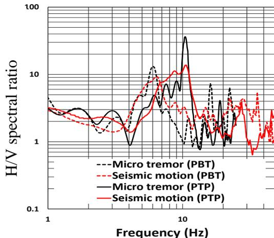
Fig. 4. Comparison of H/V spectral ratio of the seismic motion and microtremor
