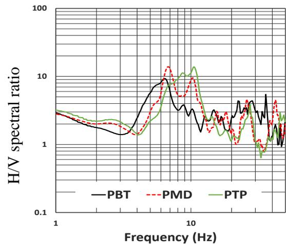
Fig. 3. H/V spectral ratio of measuring points at the pillar.
