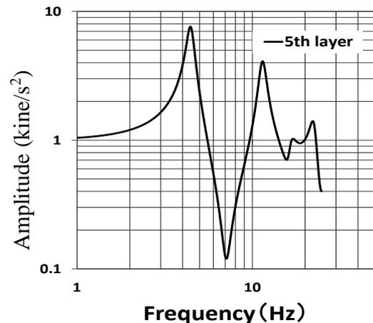
Fig. 5. Fourier spectrum of the 5th layer.
