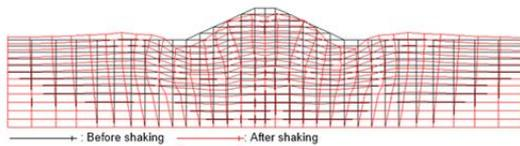
Figure 8. Deformation of the embankment (Case II)
