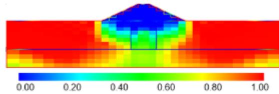
Figure 10. Excess pore fluid pressure ratio (Case II)
