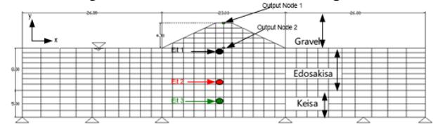
Figure 1. Analysis model and FEM mesh (Case I)
