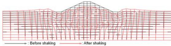
Figure 4. Deformation of the embankment (Case I)
