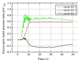
Figure 9. Excess pore pressure with time (Case II)
