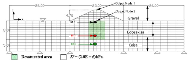
Figure 2. Analysis model and FEM mesh (Case II)
