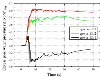
Figure 5. Excess pore pressure with time (Case I)
