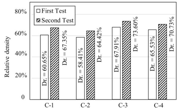
Fig. 4. Comparisons of relative density before first and second cyclic load tests
