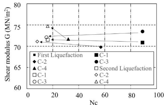
Fig. 5. Relations of  $N_c$ - $G$  between liquefaction and re-liquefaction
