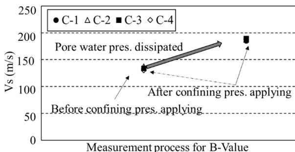
Fig. 3. Measurement of  $V_s$  with B value tests
