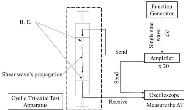
Fig. 2. Illustration of test apparatus
