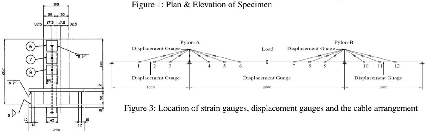
Figure 3: Location of strain gauges, displacement gauges and the cable arrangement
