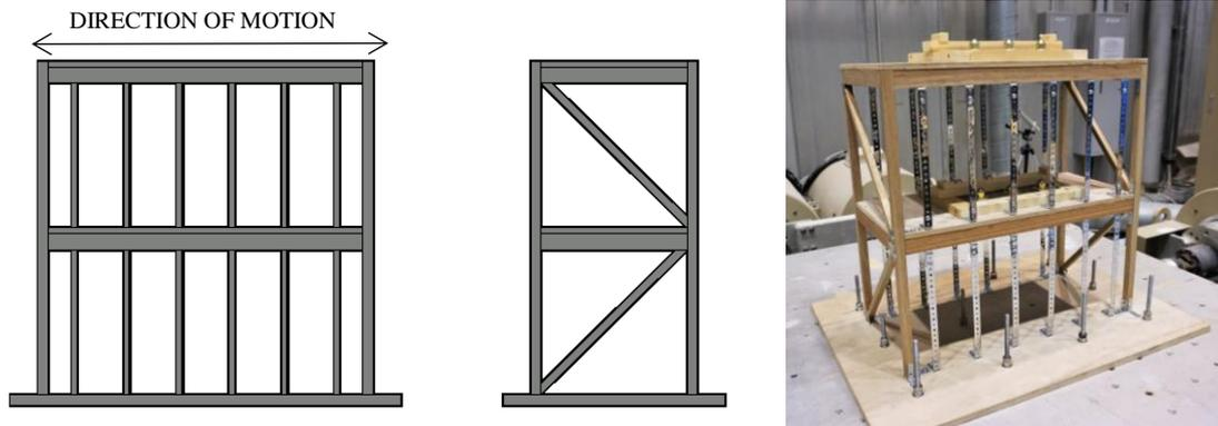
Fig. 1: Drawings of the frame design and a photo of the actual frame.
