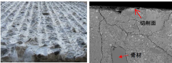
図-1 切削面例 図-2 切削断面例
