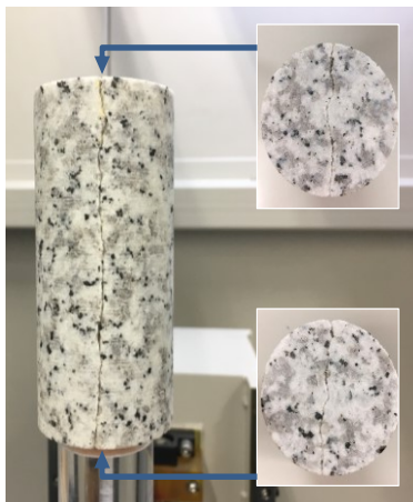
Fig.1 Cylindrical granite core of 50 mm in diameter and 100 mm in height split into two halves to create a vertical single fracture
