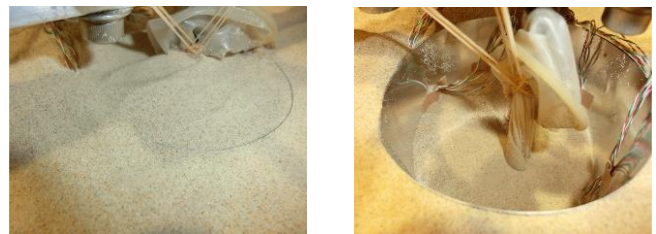
(a) Before excavation (b) After excavation Figure. 4 Experimental model before and after excavation
