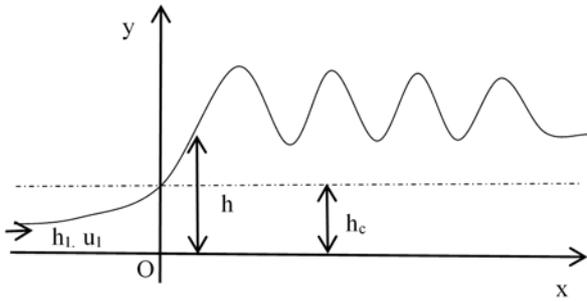
Figure 1 Sketch diagram of undular jump
