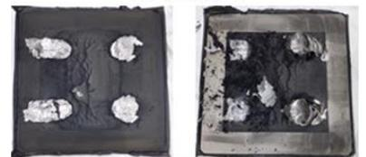
(B) 破断面上側 (C) 破断面下側
