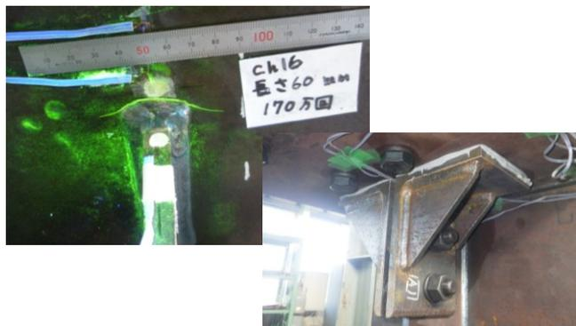
図-6 疲労き裂の一例と補強状況
