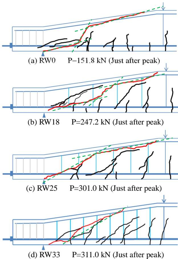
Fig. 3 Crack patterns
