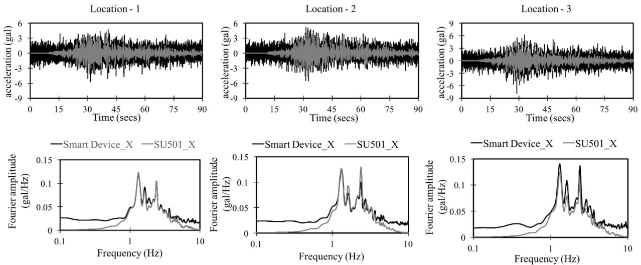
Fig. 4 Time History and Frequency Domain comparison for 017/03/02 Earthquake at 3 different location of bridge
