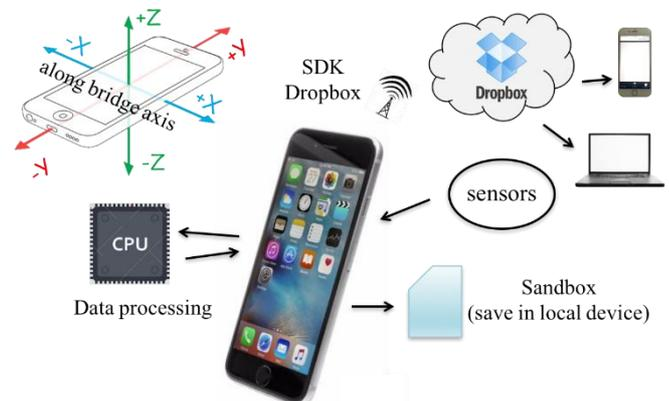
Fig. 2 Measurement system
