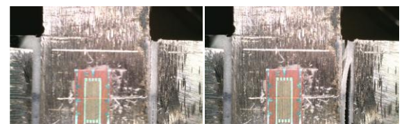
Fig. 3 Debonding image at patch plate end (E250)
